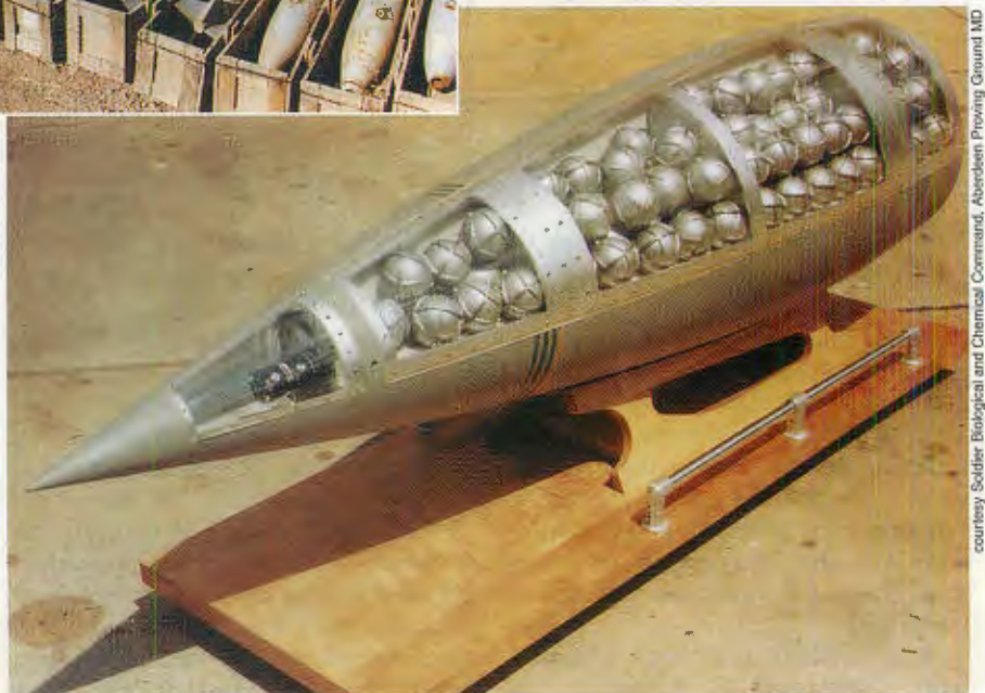
(left) UN weapons' inspectors in Iraq discovered thousands of bombs containing chemical weapons (such as these 250-kg bombs that originally held mustard gas). Many were found to be damaged and leaking in their storage areas. (below) America's 'Honest John' warhead held scores of bomblets filled with sarin nerve gas. They were designed to scatter these munitions near the intended target.
